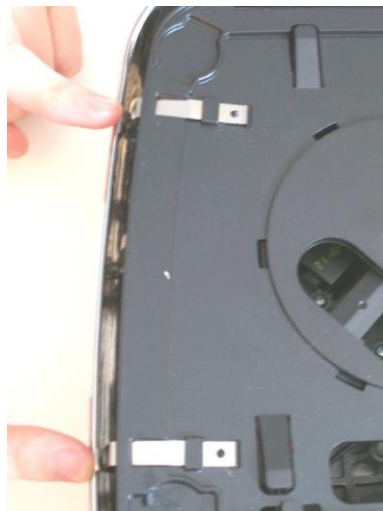
(6)- Clips installed two on each side
