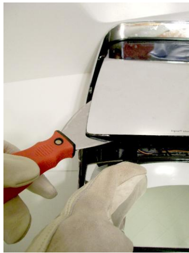
(2)-Using putty knife to loosen flat glass
