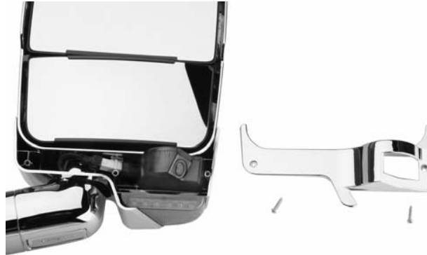
LEM with Cover plate removed
