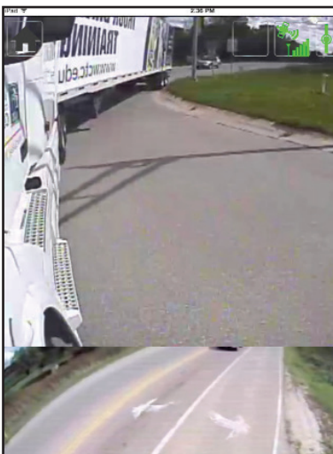
Turn signals trigger relevant iPad display for real-time blind spot viewing
